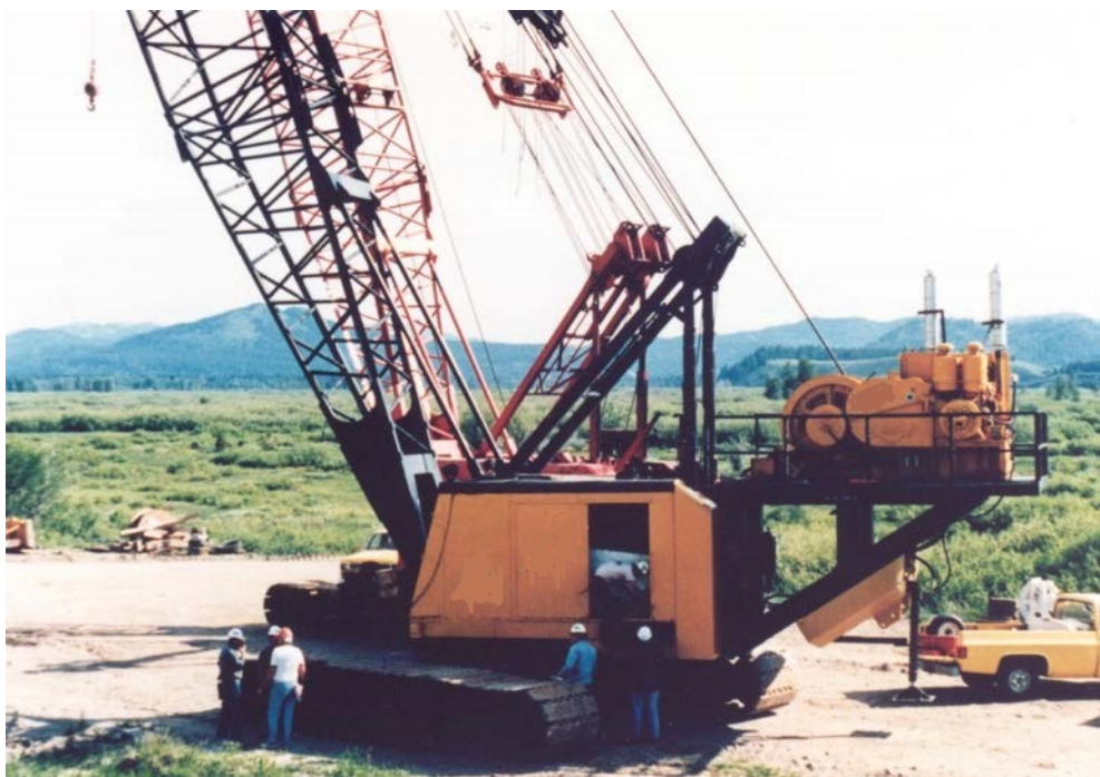
Figure 4-17. Crane with special lifting drum attached to rear of crane for use with 64 kip tamper.
