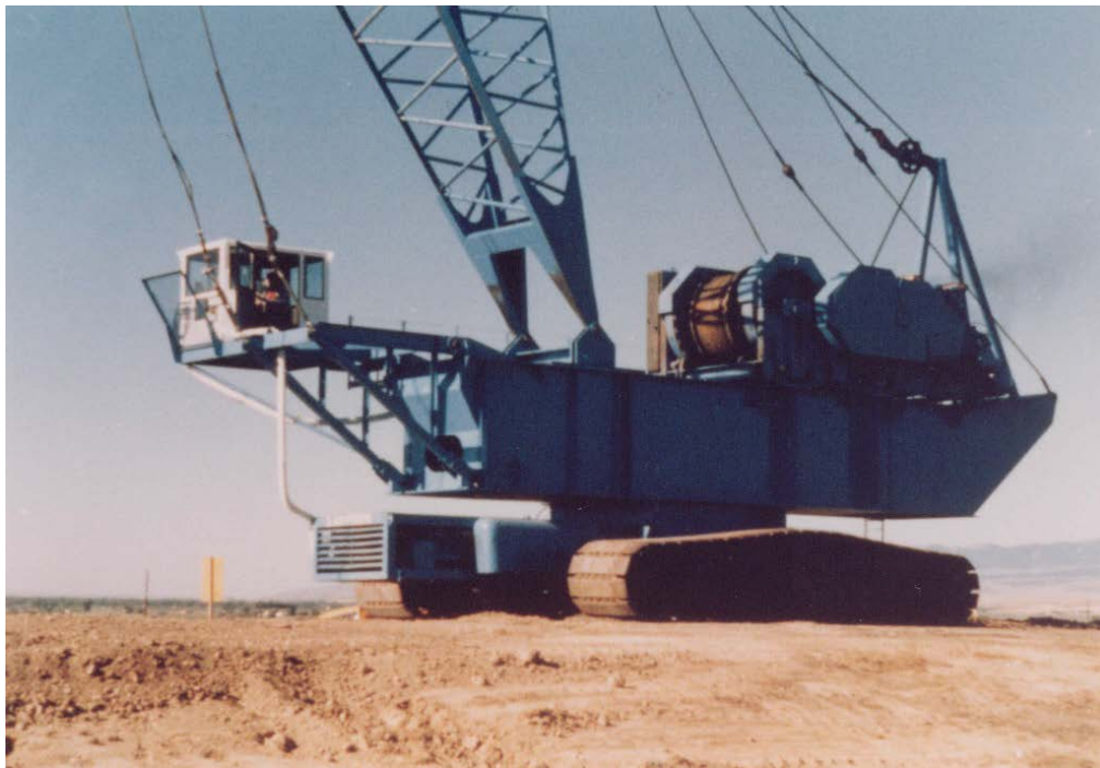
Figure 4-18. Lifting crane built only for deep dynamic compaction with 5.0-foot diameter lifting hoist and single line-rated capacity of 50 ton at line speeds of 85 feet/min used with 32 ton tampers.
