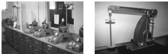
Pneumatic Type Consolidometers
