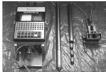
Memory chip in penetrometer. Synchronize with depth wheel & data logger at surface
