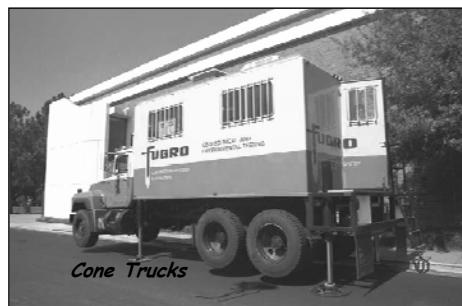
Mobile 25-tonne hydraulic pushing rigs
