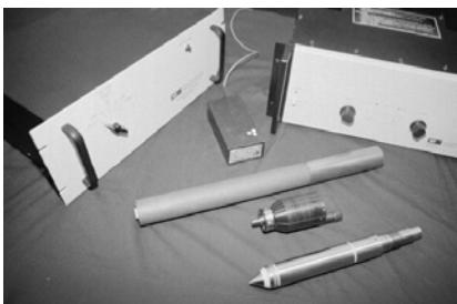
Electro-Vibrocone with Piezo-Actuator Driver and Dual-Element Piezocene Penetrometer
