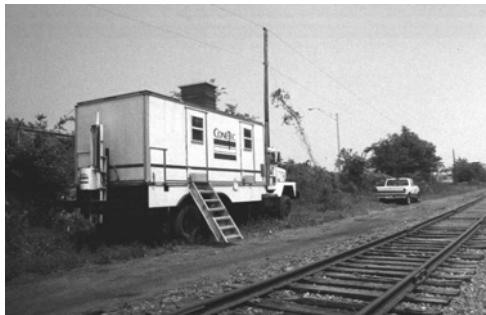
SCPTU soundings advanced by 25-tonne Cone Truck
