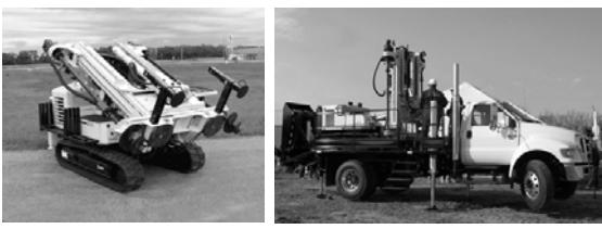
Used as a track rig      Or left on truck carrier
