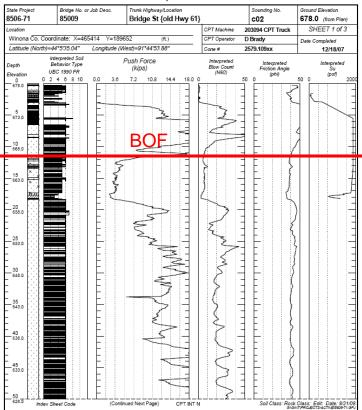
MINNESOTA DEPARTMENT OF TRANSPORTATION - GEOTECHNICAL SECTION CONE PENETRATION TEST RESULTS
